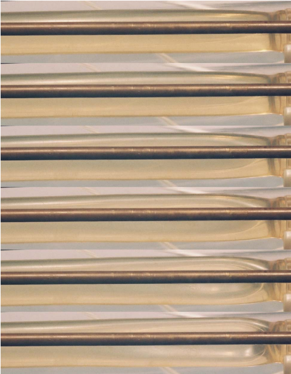
Fig. 14. Photographs of the downstream end of tube 2 at the six instants indicated in Fig. 15(b), from a viewpoint approximately in line with the minor axis of tube collapse. Flow from left to right.
