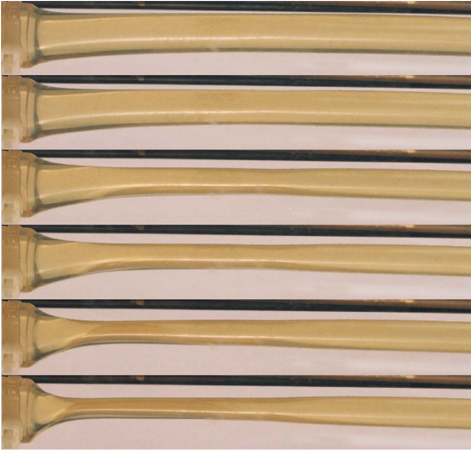
Fig. 13. The downstream end of tube 2 is photographed from a viewpoint approximately in the plane formed by the tube axis and the major axis of the collapsed cross-section, at six instants during a p_d -reduction manoeuvre as in Fig. 3. In this case, the Reynolds number was insufficient for the development of oscillation, so the tube profile was effectively static at all times. Flow from right to left. The six instants are shown in Fig. 15(a).
